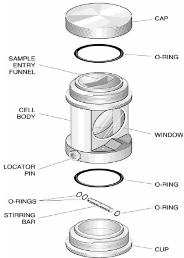
It is not necessary to take the cell apart every time there is a need for cleaning. Adding a small amount of cleaning solution and scrubbing with the swab supplied can also clean the inside of the cell.
