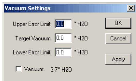
These limits must be set so that the vacuum value falls between the two limits. The vacuum LED on the front of the module will provide a guide as to which value needs to be adjusted. If the LED light is solid red, indicating the vacuum is low, adjust the Lower Error Limit to be less than the vacuum pressure reading. If the LED light is flashing red, indicating the vacuum is high, adjust the Upper Error Limit to be greater than the vacuum pressure reading.
