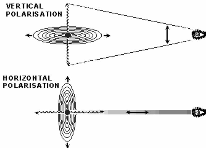
Since the PIDS signal is dependent on particle size relative to the light wavelength, valuable information about the particle size distribution can be obtained by measuring the PIDS signal at a variety of wavelengths.
