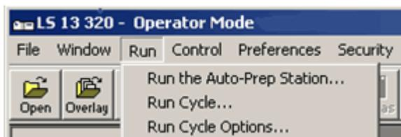
The APS is set for operation through a series of options found under the Run menu. Using these options provides flexibility in the way the APS is set up to perform analyses.
