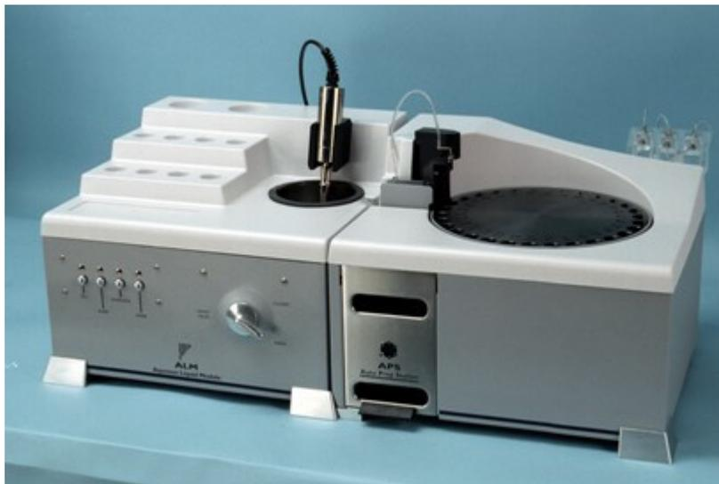
The APS adds the entire amount of sample to the ALM vessel by rinsing the sample tube into the ALM vessel with water for a preset, user-selectable time.
