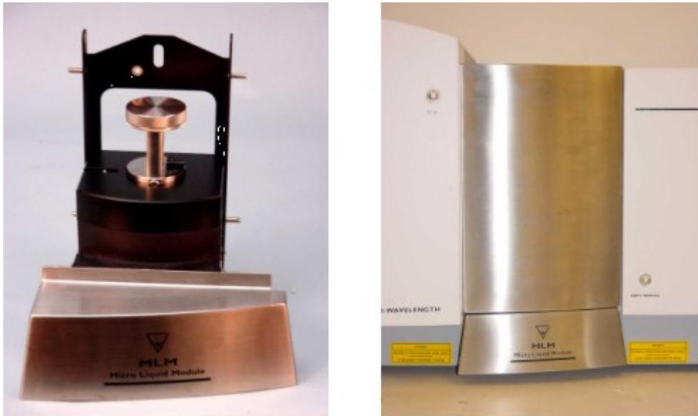
The MLM measures the entire sample in the instrument by circulating the sample with a stir bar. The amount of sample needed depends on its size and concentration. Prior sample preparation is often needed to achieve proper dispersion (see [APPENDIX B, Sample Handling](#) for more information on how to disperse samples) in order to obtain accurate and valid results.
