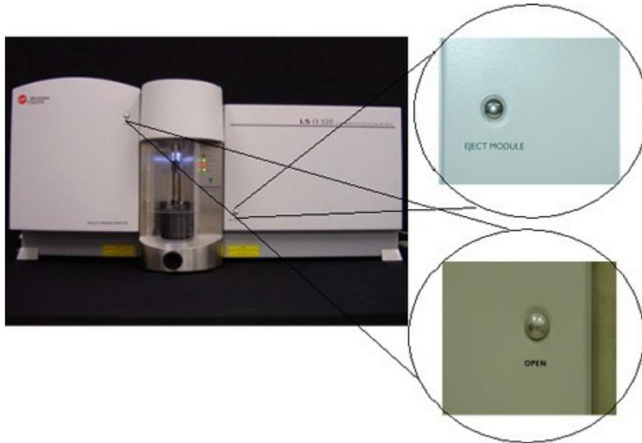
Before a module can be docked the sample cell chamber door must be retracted. This is easily done by pressing the **Open** button found on the left side of the optical bench (Figure 5).
