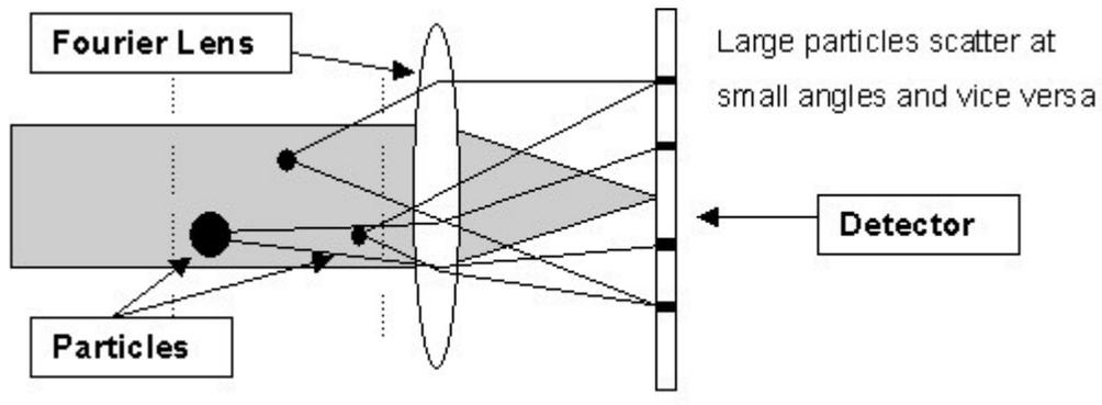
The result is that the Fourier lens forms an image of the composite scattering pattern of all particles, the pattern being centered at a fixed point in the Fourier plane. This pattern is centered at the same fixed point regardless of the position or velocity of the particle in the sensing zone.
