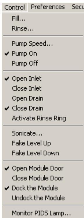
The **Aqueous Liquid Module** system can be operated through a series of manual controls accessed through software commands. These controls offer flexibility when there is a need to operate the system manually. To access these control commands:
