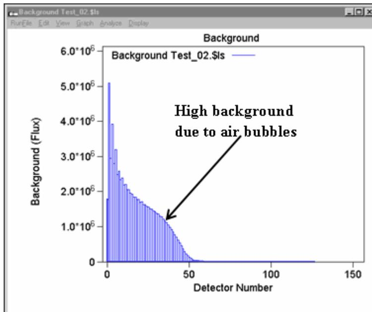
**Figure D.3** Background Showing the Presence of Contaminants
