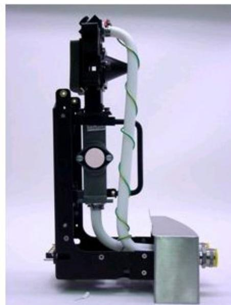
The ALM presents the entire sample to the instrument by re-circulating the sample. The amount of sample needed depends on its size and concentration. Prior sample preparation is often needed to achieve proper dispersion (see [APPENDIX B, Sample Handling](#) for more information on how to disperse samples) in order to obtain accurate and valid results.
