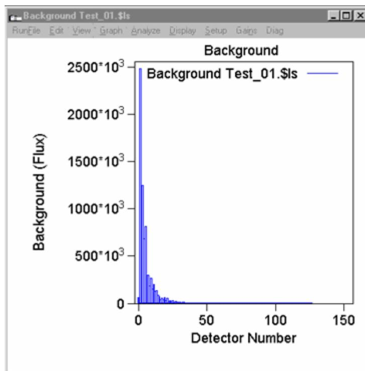
If the current background flux pattern is higher in any channel by a factor of two, the cause should be determined and remedied before running further samples. [Figure D.2](#) and [Figure D.3](#) are examples of bad backgrounds and their causes.
