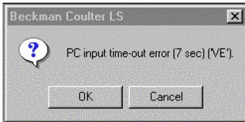
**IMPORTANT** If this occurs, ensure that an optical module is connected to the LS 13 320 bench. Make sure that the module is docking properly; otherwise contact your Beckman Coulter Service Representative. Also, check the connections between your computer and the LS 13 320 bench.
